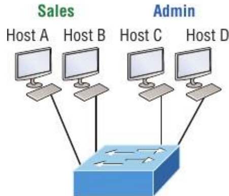
Fig 11.1 One switch, one LAN: Before VLANs, there were no separations between hosts.
